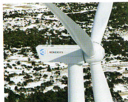
Prototype of the K100 with a capacity of 2.5 MW in Näsudden on the Swedish Baltic Sea island of Gotland.
